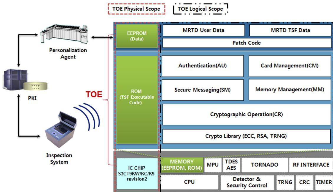
[Figure 2] Scope of the TOE
